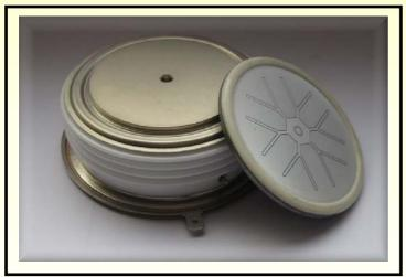
IXYS UK Westcode Ltd. announces a new pressure contact distributed gate thyristor with increased power density. This new fast thyristor with turn-off time of as little as 25µs and current rating 1605A, is symmetrical blocking with Vdrm/Vrrm equal to 2200V and therefore suitable for both voltage and current fed applications.
